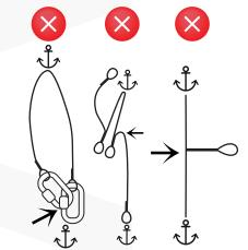
Using the lanyards in the examples shown above are dangerous and could have deadly consequences.
