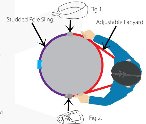
When using an adjustable rope lanyard in conjunction with the Studded Pole Sling, it must be threaded through the eye of the Studded Pole Sling (Fig 1.) and then through the connector (fig 2.).The connector gate must always be face up.
