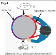
When using an adjustable rope lanyard in conjunction with the pole grip, it must be threaded through the eye of the pole grip (Fig 1.)and then through the connector (fig 2.).
