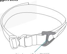
Attachment Point (EN358): Only use connectors conforming to EN362
