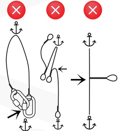
Using the lanyards in the examples shown above are dangerous and could have deadly consequences.
