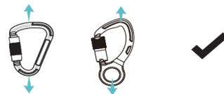
Correct loading with gate mechanism secured shut
