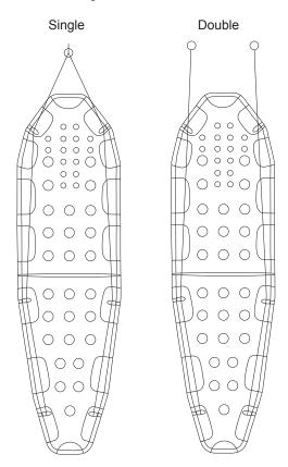
Typical vertical lift over sharp edge using double line system.
